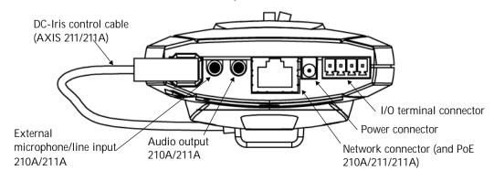
Power Connector - For connection of the PS-K power adapter (included).
